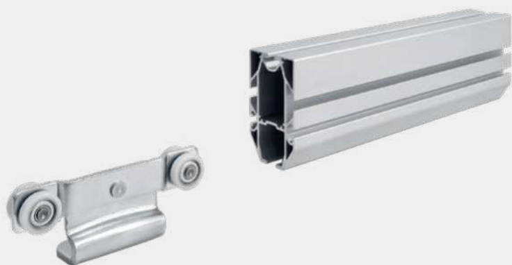
Type DL-120: Aluminium rail with roller unit for load capacity up to 800 kg per pull out rack
